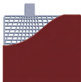
Positive plate example lead dioxide ( PbO_2 )
